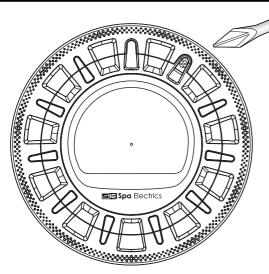
USE A SCREWDRIVER TO LOOSEN THE CAPTIVE SCREW
