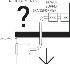
**2B:** IF THE TRANSFORMER DOES NOT MEET THE REQUIREMENTS, IT WILL REQUIRE REPLACEMENT
