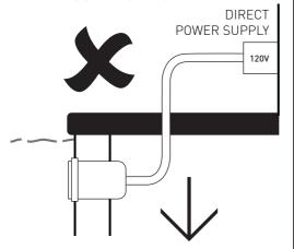
**1B:** A 12V AC TRANSFORMER **MUST** BE INSTALLED BETWEEN THE 120V POWER SUPPLY AND POOL LIGHT
